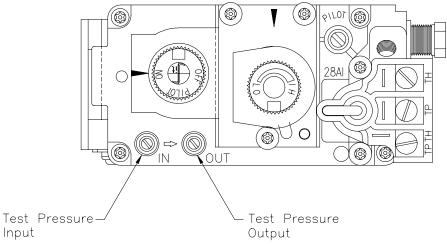
FIGURE 7. Pressure Test Point Location
